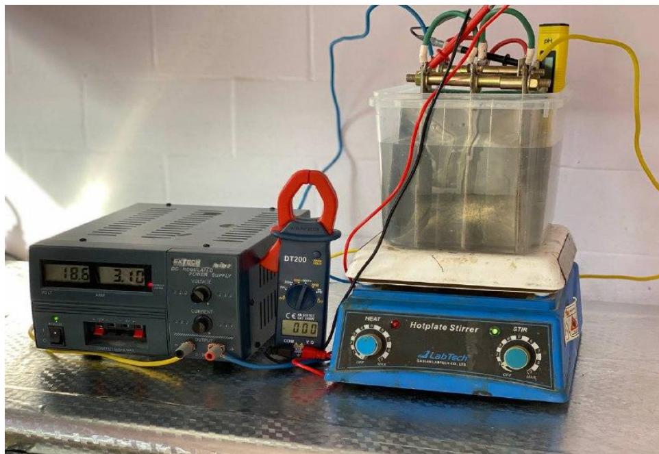
Image 3: Electrocoagulation's apparatus setup.
