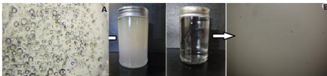
Fig. 7 Microscopic and photographic images of oil/water mixture before A and after B separation
