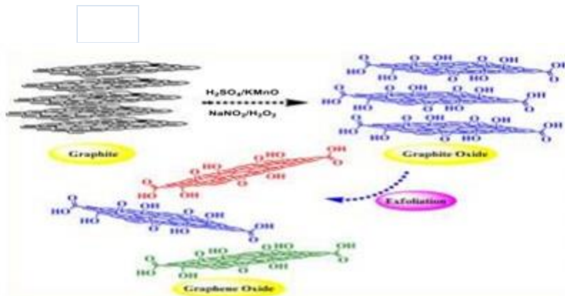
Figure (3): Mechanism of the prepared of graphene oxide (GO)
